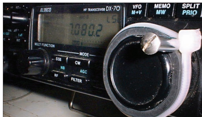
● Fig. 1: The simple - yet effective quick-tune handle for rigs that don't have one as standard (See text for more detail).
