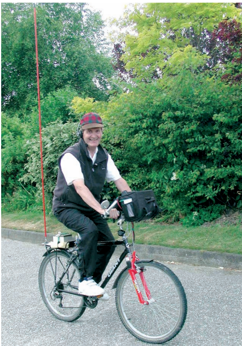
● A lightweight antenna for bicycle mobile based on a large Firestik antenna, modified for use on the 28MHz band. The antenna is mounted on an aluminium plate fixed to the bike carrier.
